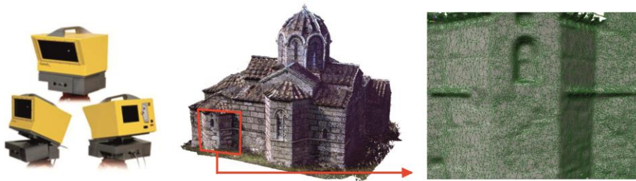
Production of a 3D model from Terrestrial Laser Scanning
